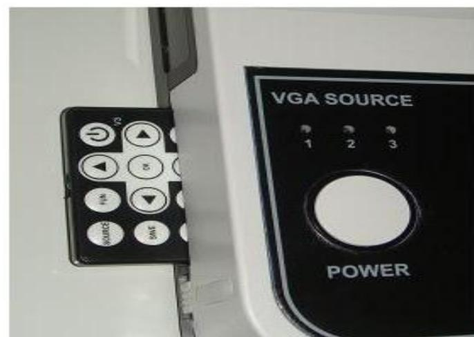
7. Finish using, power off (Indicator light is off), disconnect power cable, put down the arm lamps, put down the lens pole and lightly push camera, put down the stand, to keep the document camera in a good condition.
